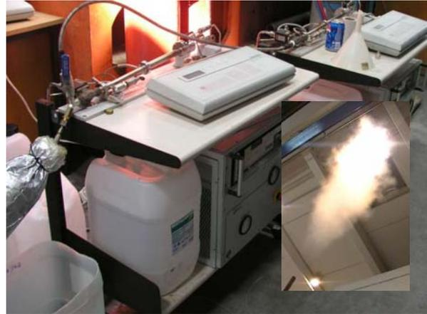
Fig. 3: Hydronic 2x15kW H<sub>2</sub>/O<sub>2</sub> Steam Generator in the parallel mode. Exhaust of superheated steam.
