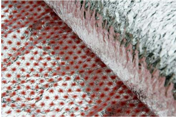
Figure 2: The new flock insulation shows low weight and thermal conductivity paired with unmatched reversible compressibility.
