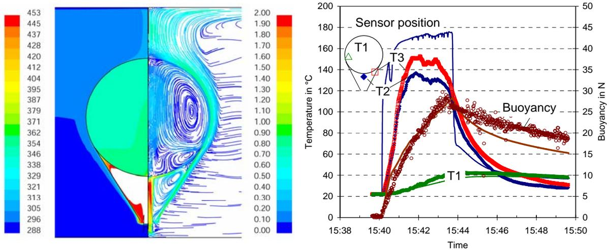
**Figure 4: Simulated temperature distribution ( $^{\circ}\text{K}$ ) and streamlines colored by velocity magnitude (m/s) (left), comparison of simulated and measured values of temperature and lift during a heating/cooling maneuver (right).**
