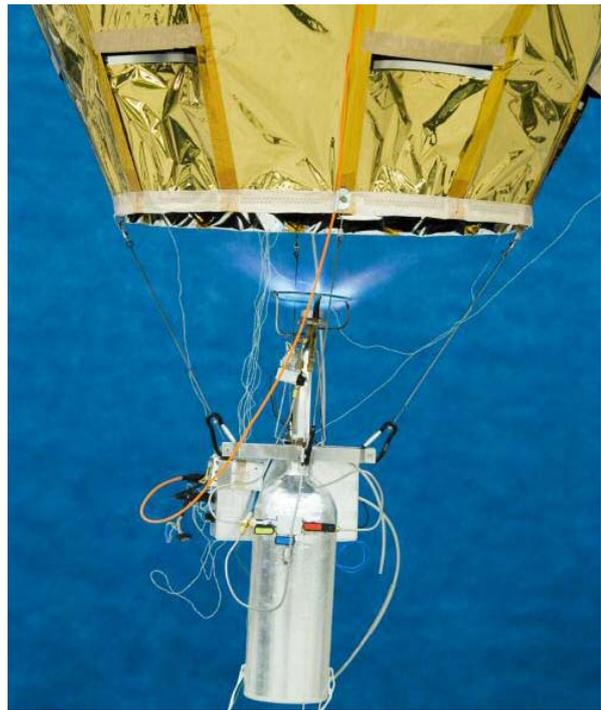
**Figure 3: Gondola with onboard computer and swirl burner.**
